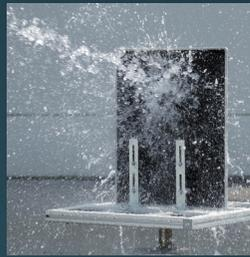
Structured to prevent the infiltration of liquids, FDR D-EVO III conforms to IPX6 standards and can withstand jets from any direction\*. There is no need to worry about fluid penetration from cleaning or body fluids. FDR D-EVO III also complies with IP5X for dust-proof protection, preventing infiltration of small particles\*.
